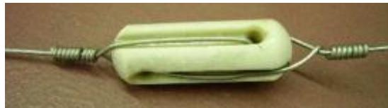
I read more. Turns out, insulators are critical. They isolate the antenna from ground. We'd missed that. Our wires were attached directly to the tin roof. We had one insulator at the mast, but nothing at either end of the wire.
